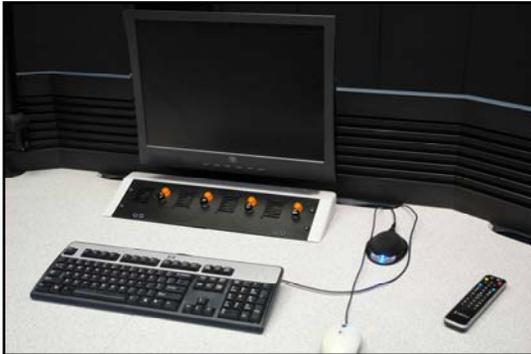
We've added a slatwall to mount the touch screen and other monitors on ergonomically adjustable articulating arms. The radio panel is integrated into a low-profile desktop turret that sits underneath the monitors.
