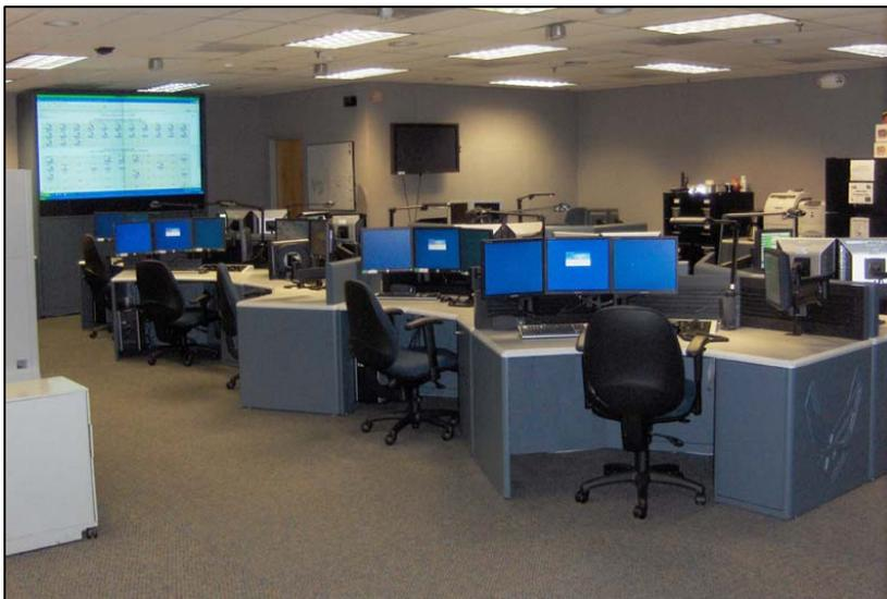
more functional furniture. In order to do that, the new consoles had to be able to accommodate all of the communications equipment from the legacy furniture. The migration from old to new has to be performed by Siemens technicians and includes a touch screen, a CPU, a large punch down wiring block and a rack-mounted speaker panel.
